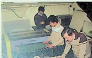
Aluminum plates for the 6 presses are burnt on sophisticated equipment.
